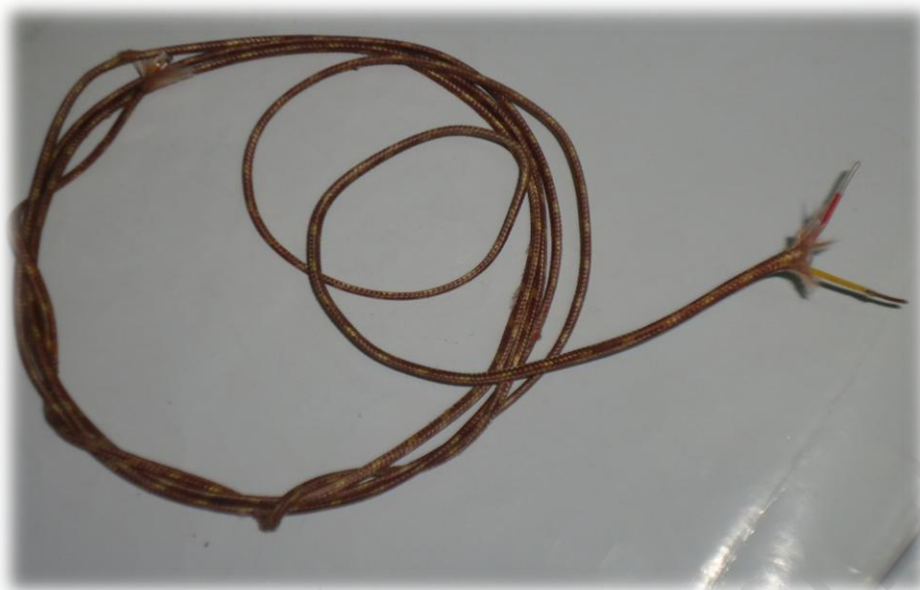
Fig 4.3 the K type thermocouple
