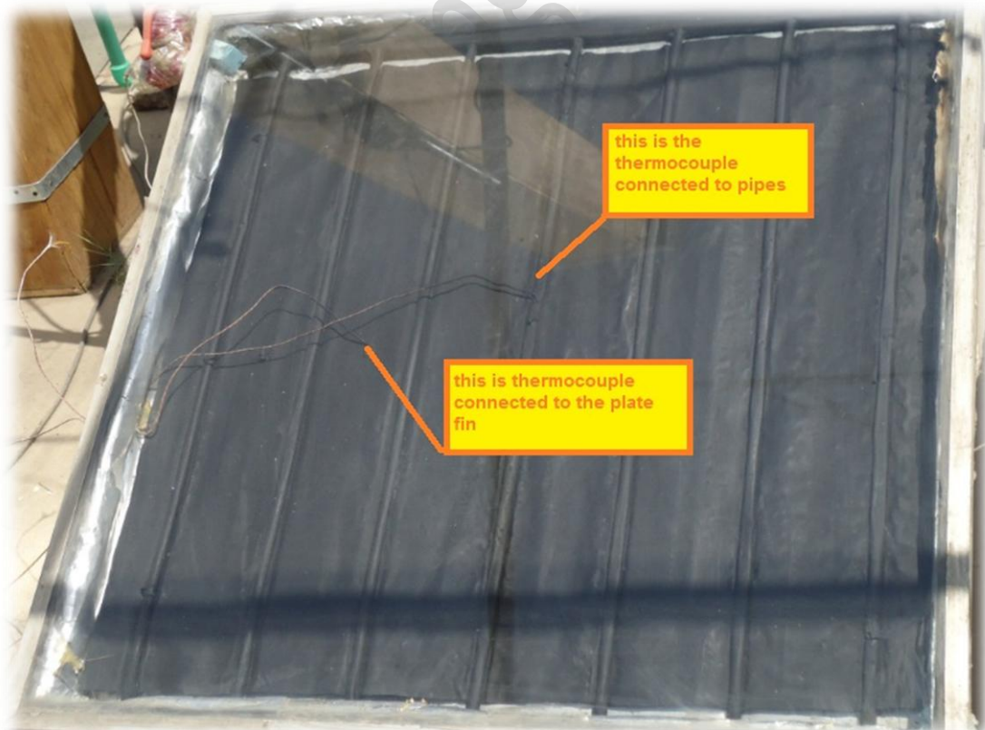
Fig 4.7 thermocouples on the absorber
