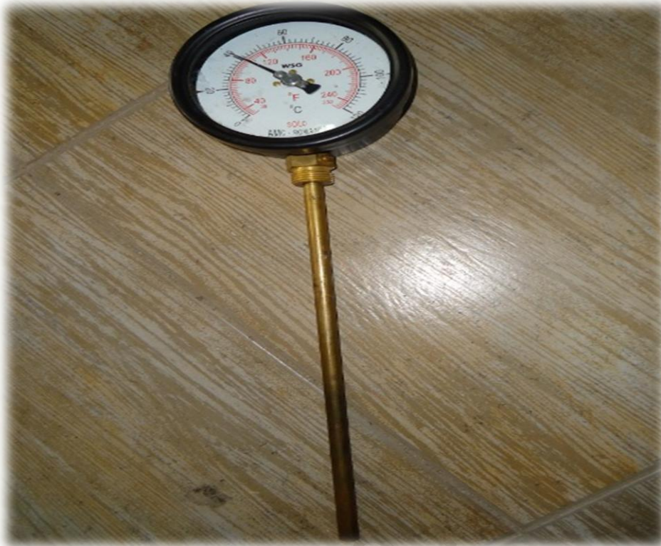
Fig 4.8 the thermometer used inside storage tank
