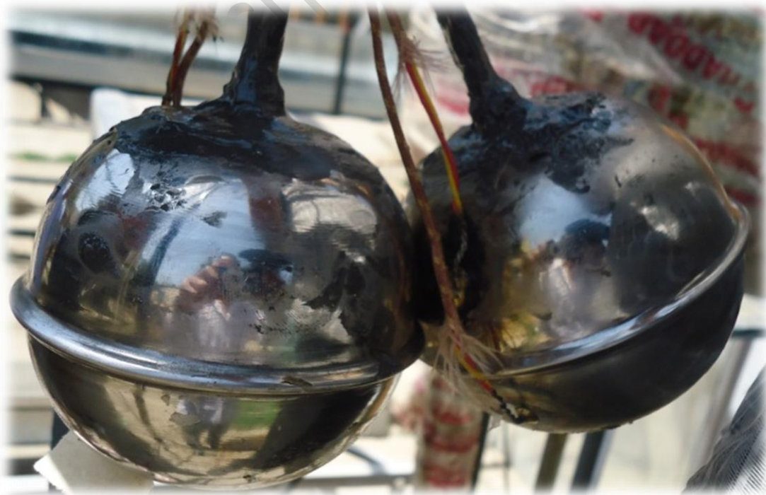
Fig 4.9 thermocouples on outer surface of PCM capsules
