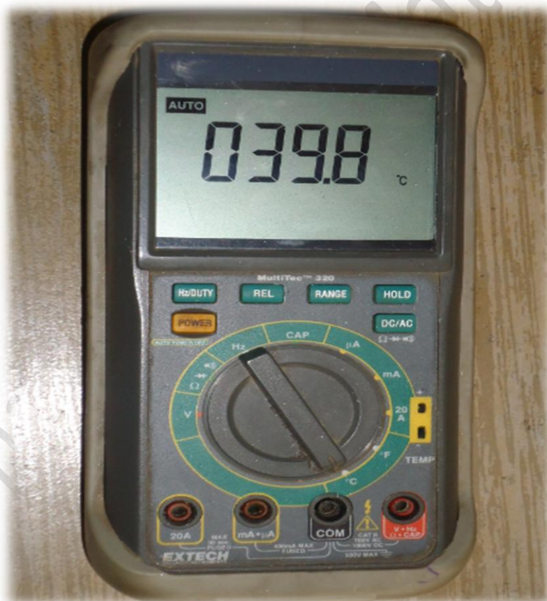
Fig 4.4 the voltmeter used to measure the temperature using thermocouple
